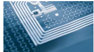
RFID tags with chip and aerial
